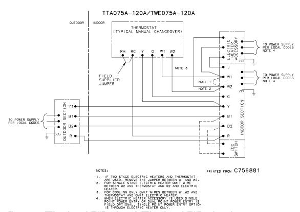
Figure 11. TTA090A, 120A/TWE090A, 120A; TTA075A, 100A/TWE075A, 100A
